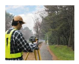
The world's first "Rock-and-Read" technology provides an additional survey style option that allows a rod person to rock the staff back and forth, instead of keeping the staff plumb.
