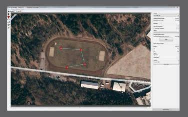
Flight planning is simple, much is contained in the Mobile Ground Station firmware. Simply enter your required parameters to survey your area of interest right at the project site. Flight pattern and attitude are automatically optimized and defined by your settings.
