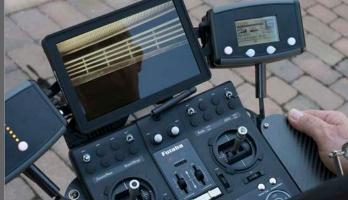
View real-time data on the monitor of the Mobile Ground Station or using the video goggles. Freely adjust the Falcon 8's alignment and image zoom using the live image.
